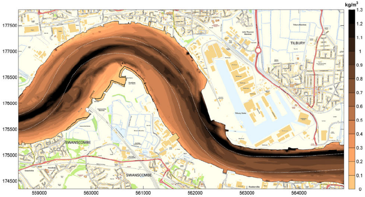
Figure 4.16: Maximum depth averaged suspended sediment concentration, Option B
